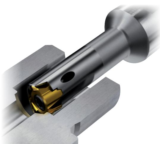
Innovative tool system for boring applications in bores from  $\varnothing$  7.8 mm on, consisting of triple-edged indexable inserts with different cutting edge geometries as well as anti-vibration solid carbide shanks or steel shanks with internal coolant supply.
