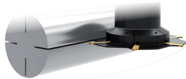
simmill H2 provides very high process reliability and tight axial and radial runout tolerances thanks to precision ground two-edged indexable cutting inserts in combination with an active and easy-to-use clamping system. Maximum possible cutting depth up to 18,0 mm with a cutting diameter of 100,0 mm.
