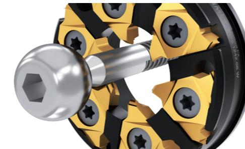
Tool group for thread whirling applications in medical technology, general massproduction as well as with „difficult-to-machine materials“. System contains of highly precise indexable carbide inserts with three cutting edges with selected grades and a variety of matching whirling rings for different machines and driven units.
