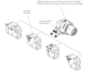
System of modular basic toolholders and matching cassettes for a variety of simturn product groups. The basic toolholders with polygonal shanks according to ISO 26623 are available for internal and external applications.
