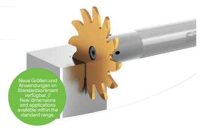
Six-edged milling inserts for general groove milling with cutting diameter Ø 28 mm and cutting edge widths from 1,2 mm to 2,5 mm as well as 12-edged cutting inserts for groove, slot and parting off milling with milling depths up to 16.5 mm and cutting edge widths from 0,5 mm to 6,0 mm! A high-performance toothing ensures high torque transmission and a long service life with maximum flexibility.
