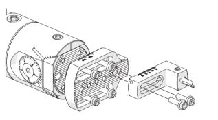
Modular tool system including cassettes for using the standard simturn product groups simturn AX and simturn DX as well as compatible adaptors for fine turning heads.
