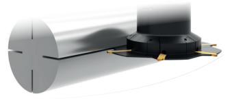
simmill H2 provides very high process reliability and tight axial and radial runout tolerances thanks to precision ground two-edged indexable cutting inserts in combination with an active and easy-to-use clamping system. Maximum possilble cutting depth up to 18,0 mm with a cutting diameter of 100.0 mm.
